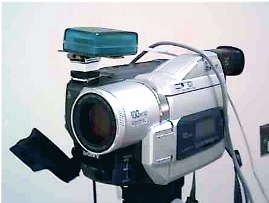
Figure 6. Digital Video Camera-system attached GPS-Receiver
