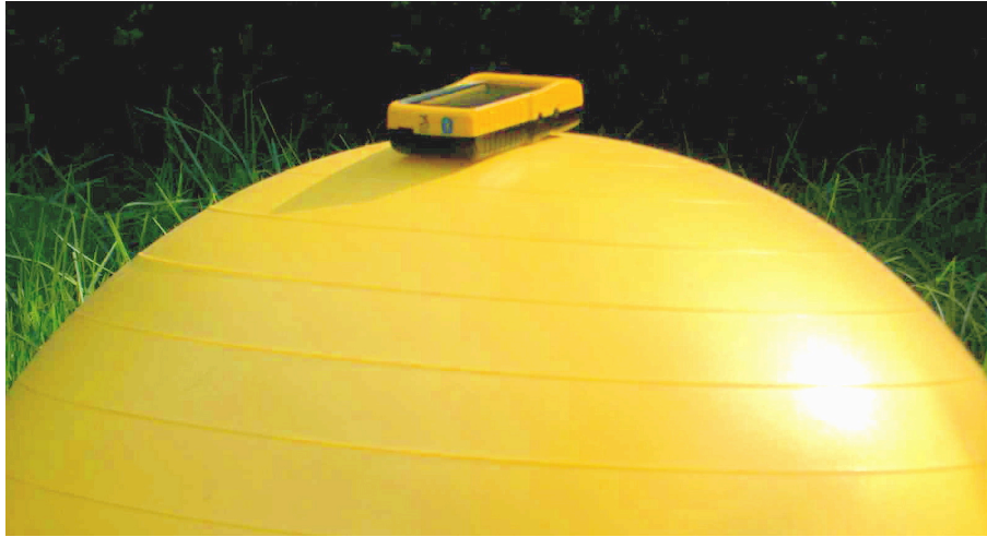
Figure 7. Marker Ball with attached wireless GPS-Receiver.
