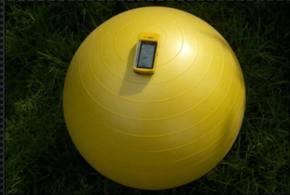
Marker ball with attached Bluetooth GPS- receiver
