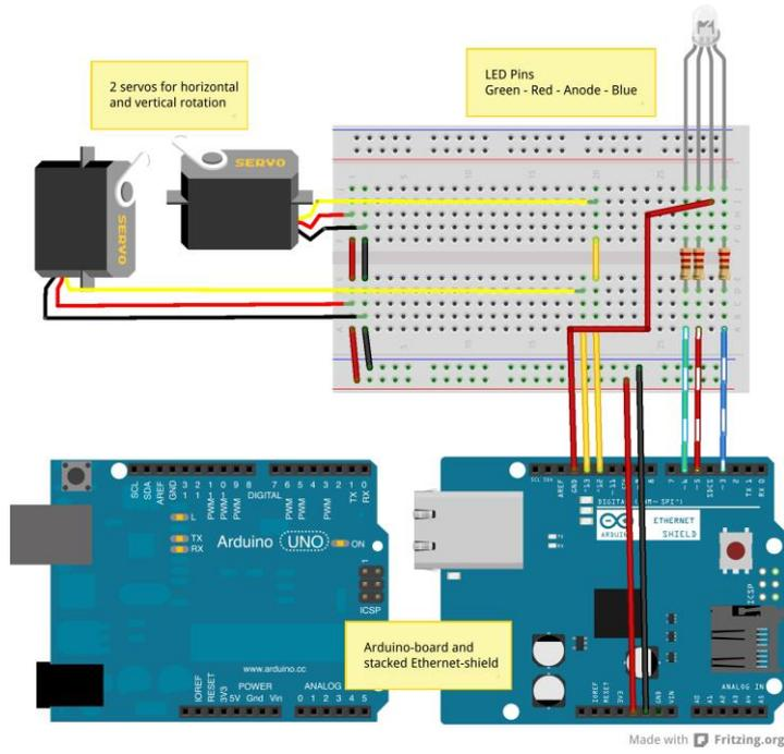
Figure 10. Schematic view of a single lighting unit.
