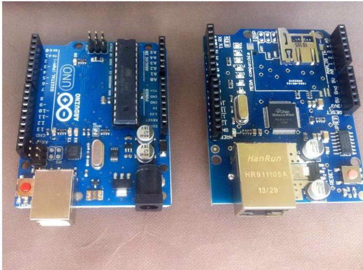
Figure 7. Micro-controller board and Ethernet shield
