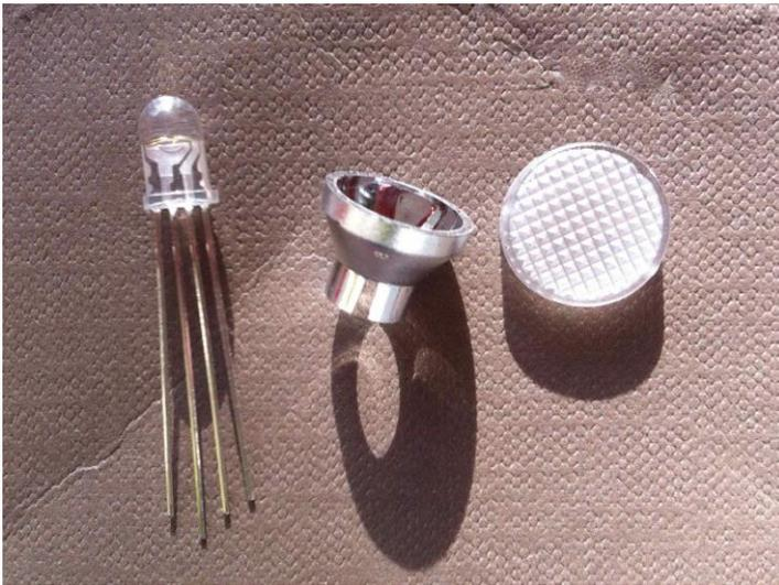
Figure 2. RGB-LED, reflector and diffusor.
